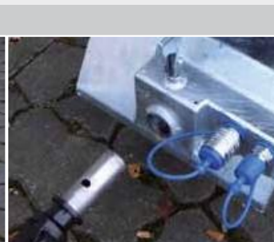
Hitch system and double-acting hydraulic connector, standard
