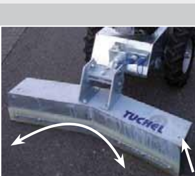
Double-lip manure scraper incl. levelling and interceptors
